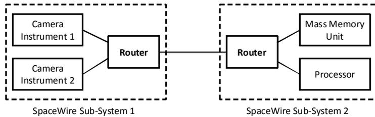
**Figure 1: Example SpaceWire network containing two distinct sub-systems**
