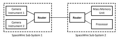
Figure 1: Example SpaceWire network containing two distinct sub-systems
