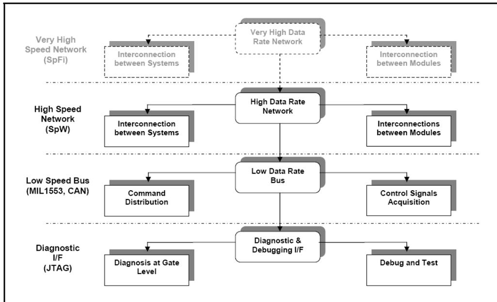
**Figure 1. Avionics network and bus hierarchy**
