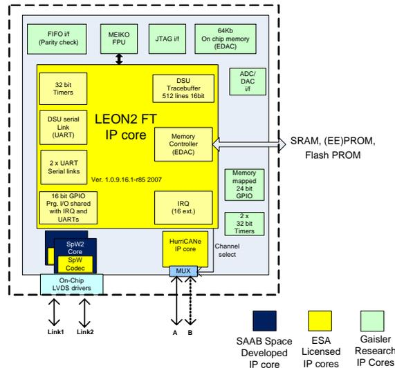
**Figure 2. RTC architecture**
