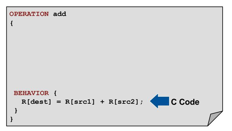
OPERATIONs are used to describe the behavior of functional units in the processor.
