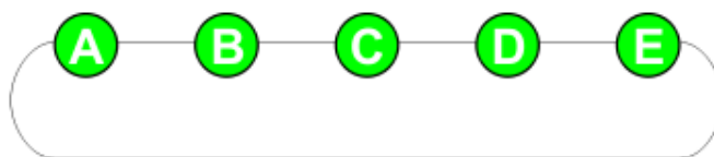
Figure 6.5 - a ring-connected set of nodes
