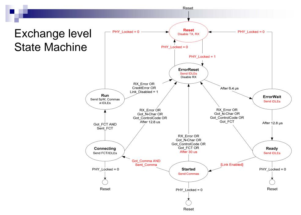
**RX\_Error** = Disconnection error OR Decoder error [Link\_Enabled] = (NOT Link\_Disabled) AND (Link\_Start OR (Auto\_Start AND Got\_Comma))
