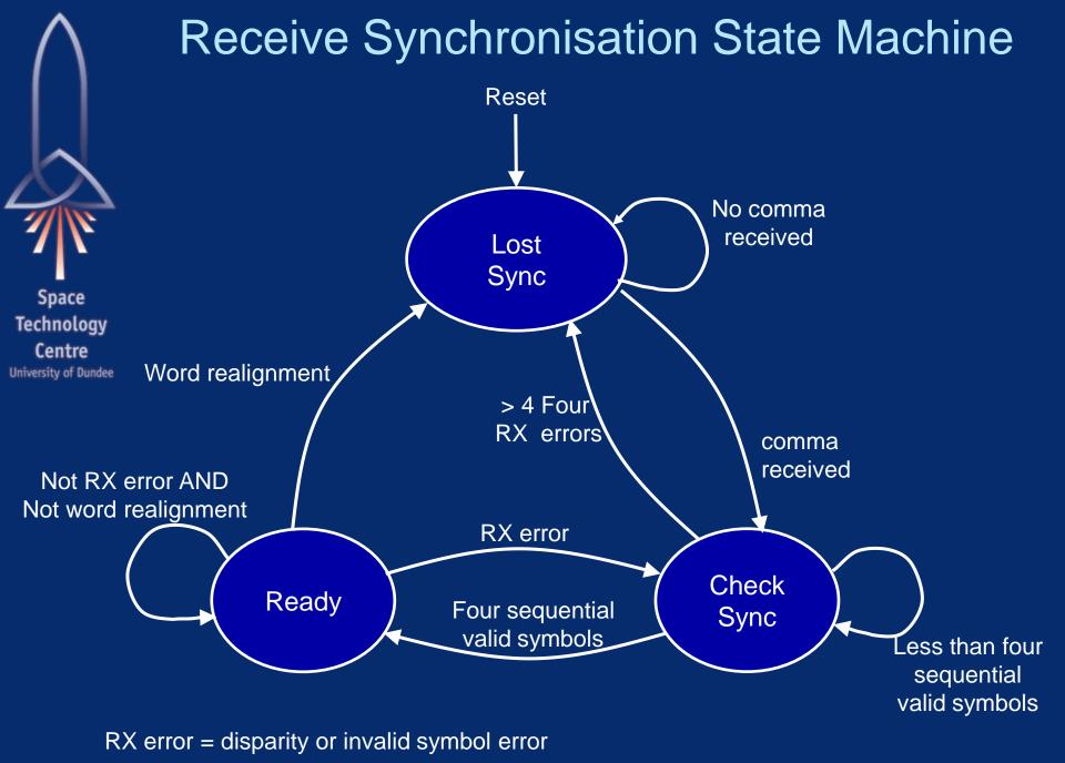
Word realignment = word synchronisation lost (i.e. comma in position other than LS byte)
