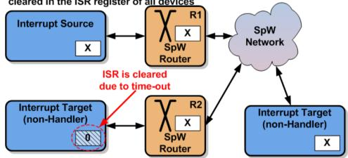
The Interrupt Acknowledge will propagate in the network until it reaches a router in which the timeout for the specific interrupt identifier has expired
