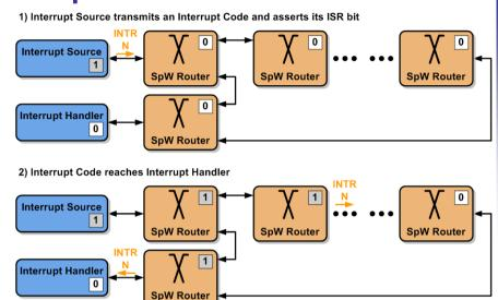
3) The Interrupt Handler responds quickly, before the Interrupt Request has reached the farthest router in the network
