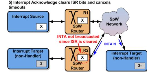
6) After all timeouts have expired, the specific ISR bit is cleared in the ISR register of all devices
