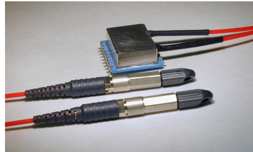
SpaceFibre transceiver module with Diamond AVIM connectors
