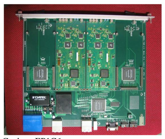
8 ch analog input FADC mezzanine card is developed at KEK (FINESSE format)
