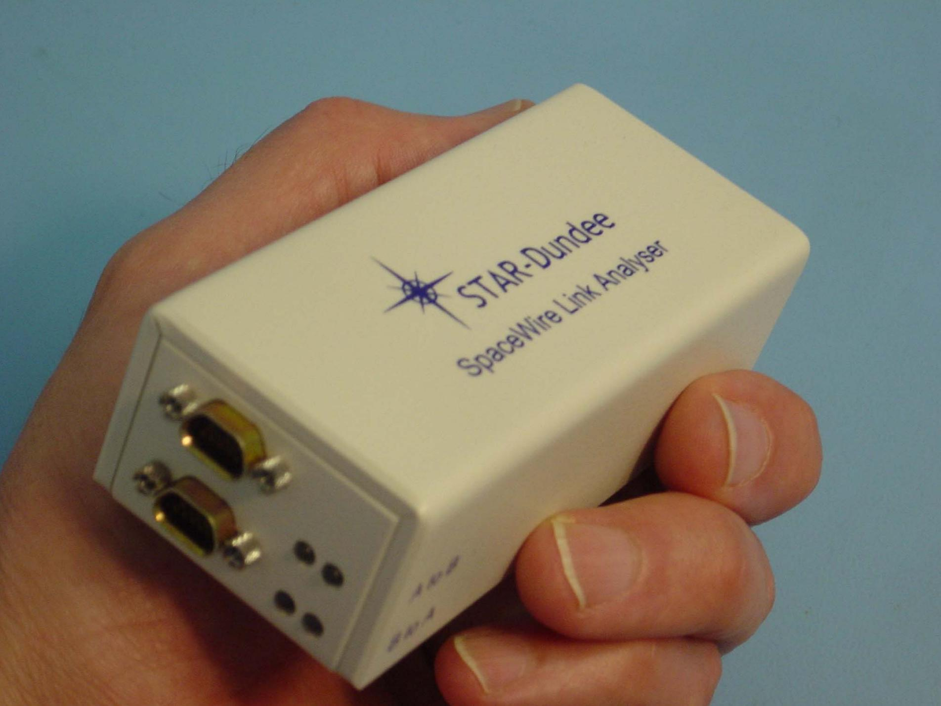
A hand is holding a small, white, rectangular electronic device. The device has a blue logo of a starburst with a central dot. To the right of the logo, the text 'STAR-Dundee' is printed in a blue, sans-serif font. Below this, 'SpaceWire Link Analyser' is printed in a smaller, blue, sans-serif font. On the left side of the device, there are two gold-plated connectors, likely SpaceWire ports, and several small circular holes. The background is a plain, light blue surface.
