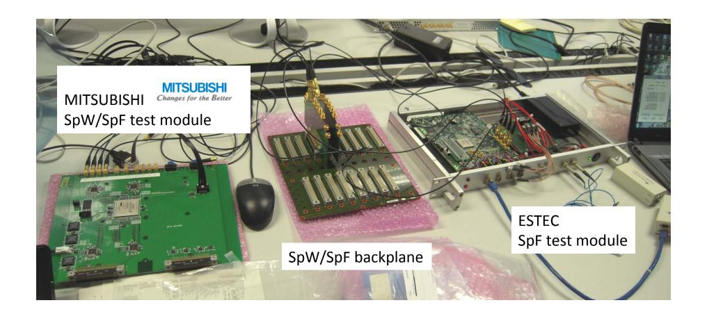
SpaceFiber connectivity test at ESTEC on 22/02/2010
