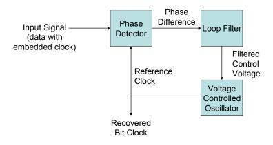
Figure 3-4 Typical Phase-Locked Loop
