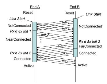
Figure 3-17: Initialisation through FarConnected State
