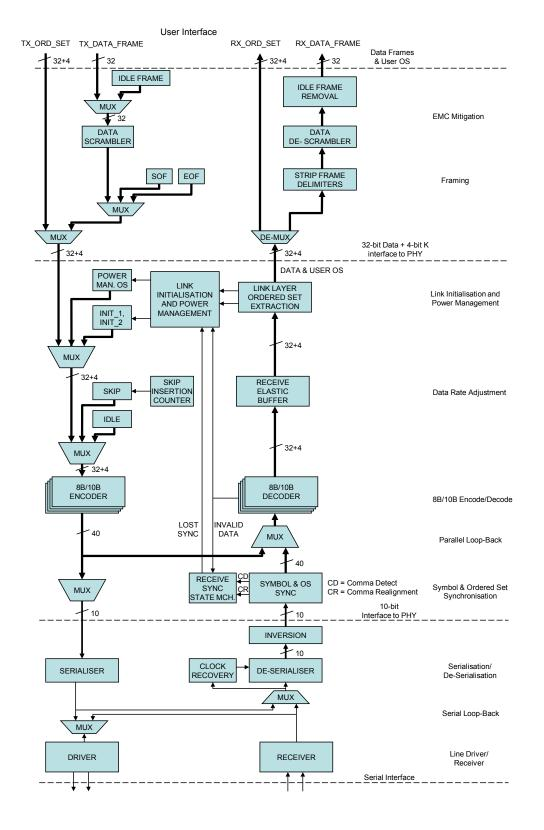
Figure 2-2 SpaceFibre CODEC Architecture
