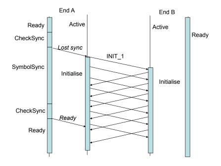
Figure 3-19: Re-Initialisation after Loss of Sync
