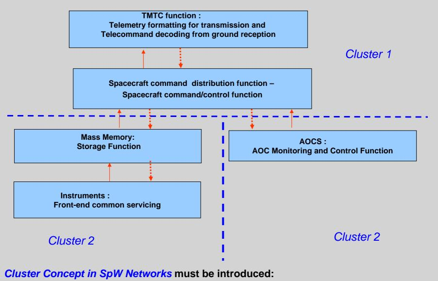
Example: Central Computer, AOCS, MMS & PayLoad servicing
