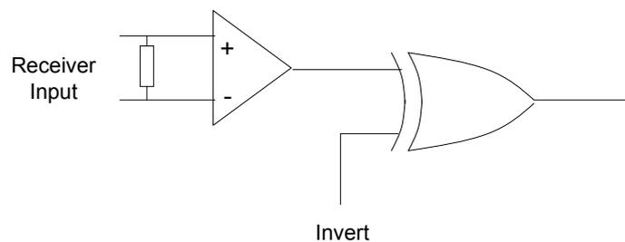
**Figure 3-20: Inversion of Receiver Input**
