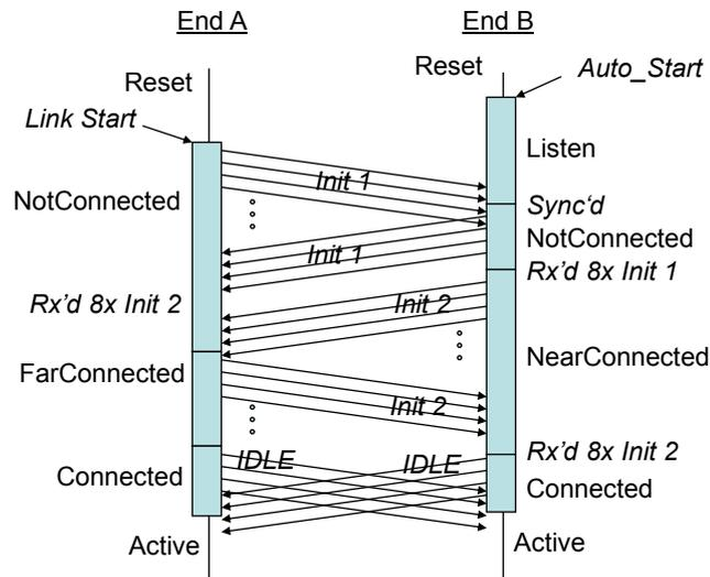
Figure 3-15: Initialisation from Auto-Start through FarConnected State
