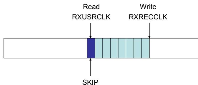
**Figure 3-9 Receive Elastic Buffer Emptying**
