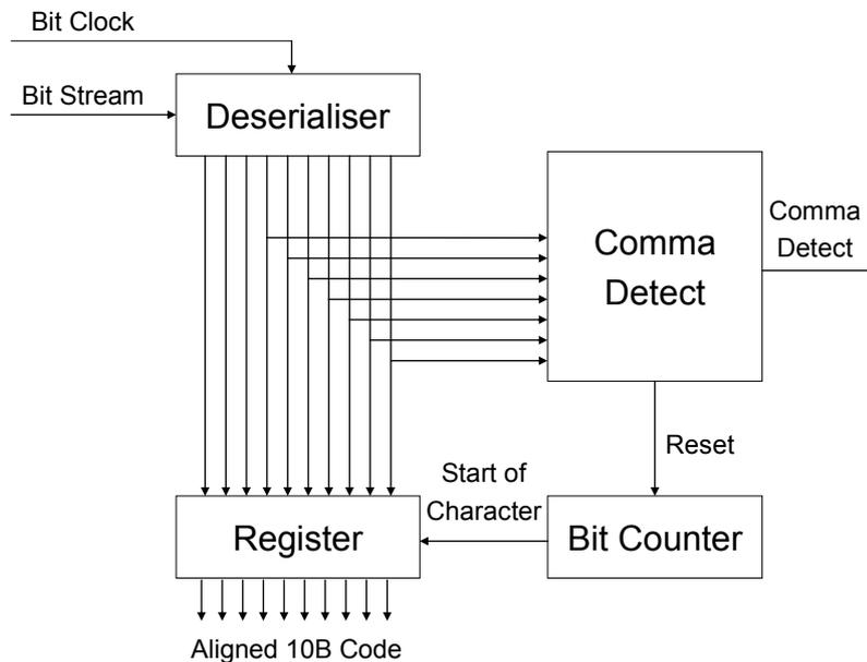
**Figure 3-7 Character Alignment During De-serialisation**
