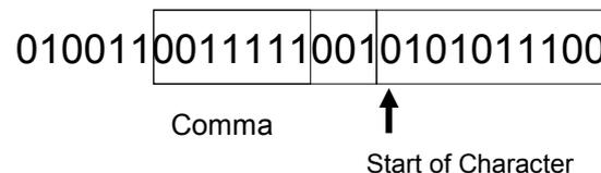
**Figure 3-5 Character Synchronisation Using a Plus Comma**
