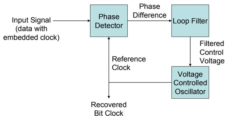
**Figure 3-4 Typical Phase-Locked Loop**
