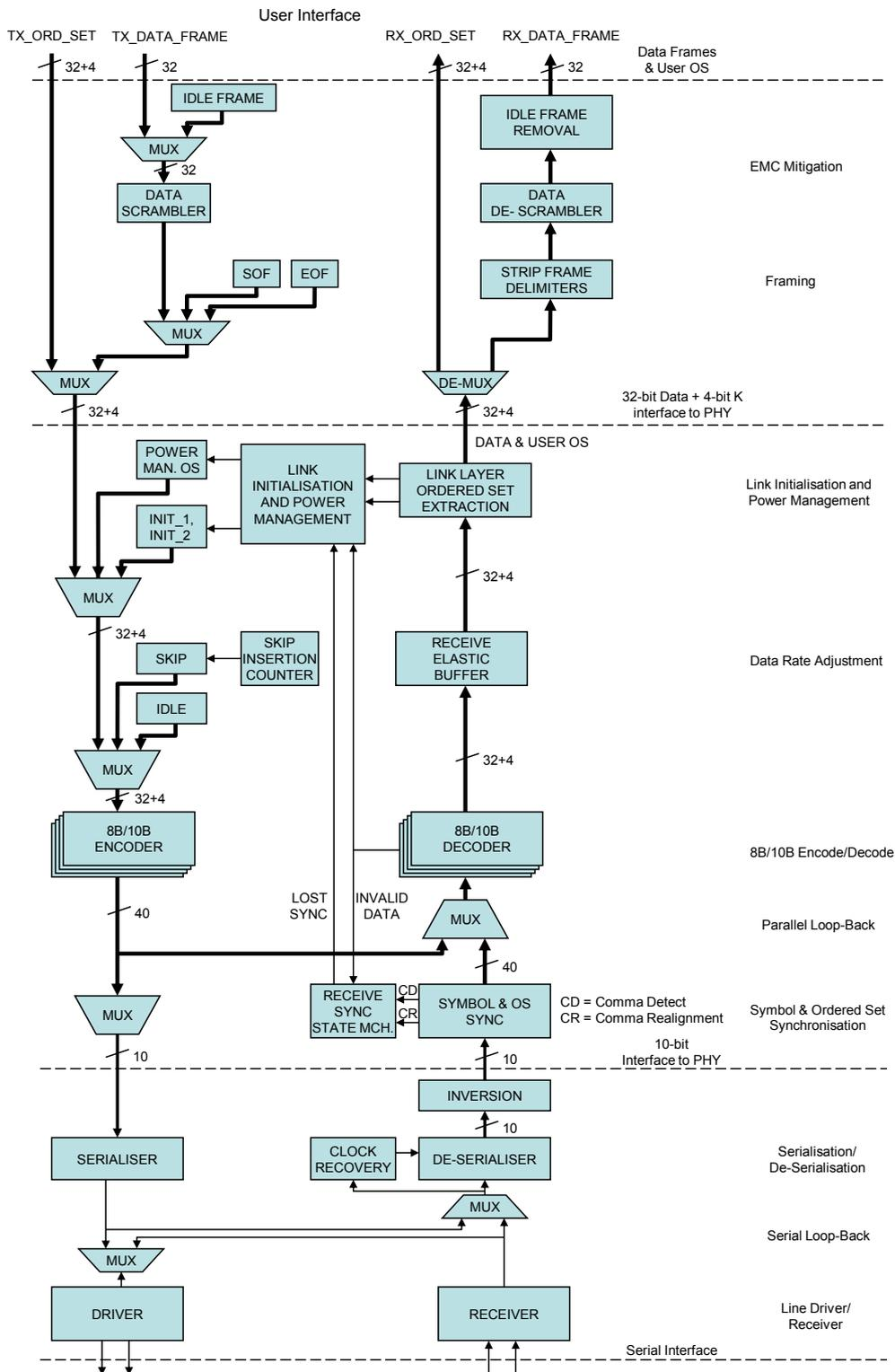
Figure 2-2 SpaceFibre CODEC Architecture
