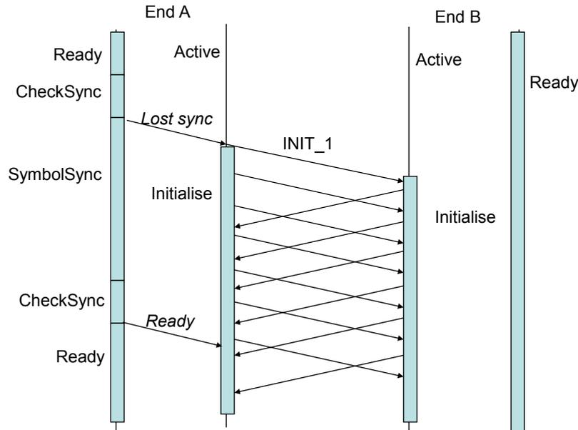
**Figure 3-19: Re-Initialisation after Loss of Sync**
