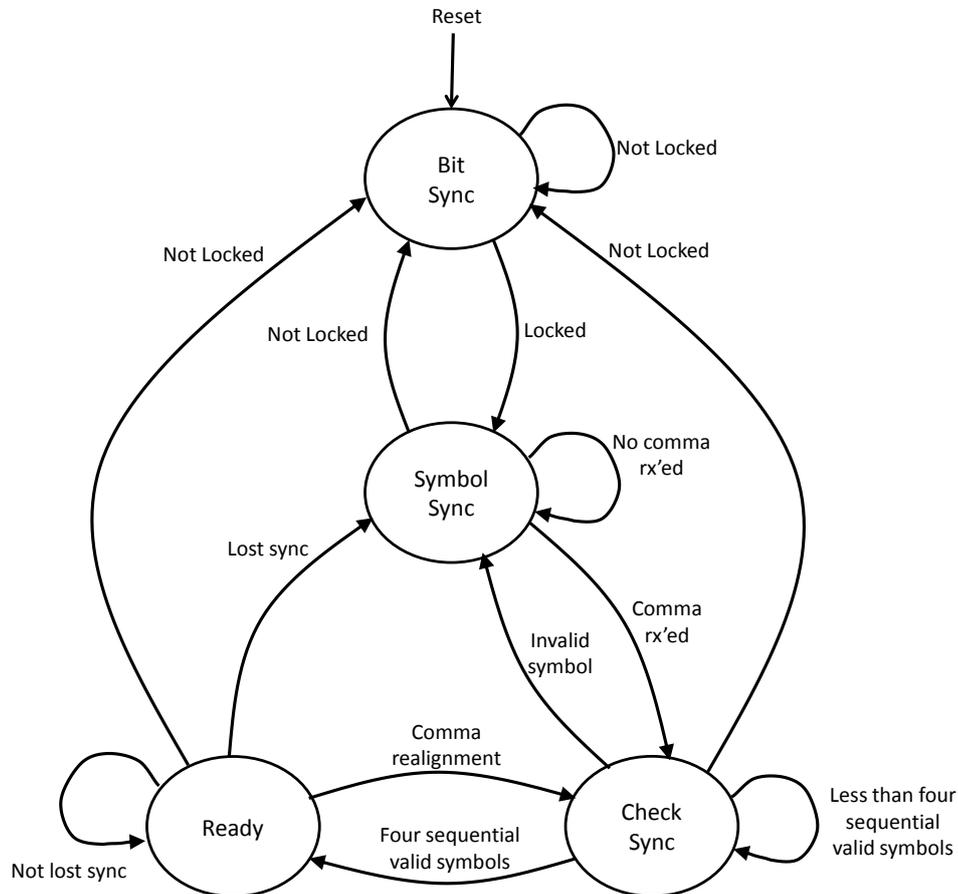
**Figure 3-11 Receive Synchronisation State Machine**
