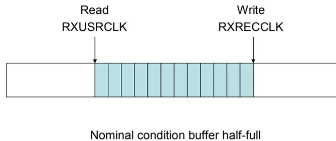
**Figure 3-8 Receive Elastic Buffer - Nominal Condition**
