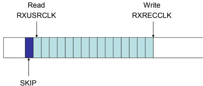
**Figure 3-10 Receive Elastic Buffer Filling Up**
