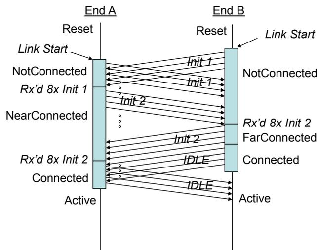
**Figure 3-17: Initialisation through FarConnected State**
