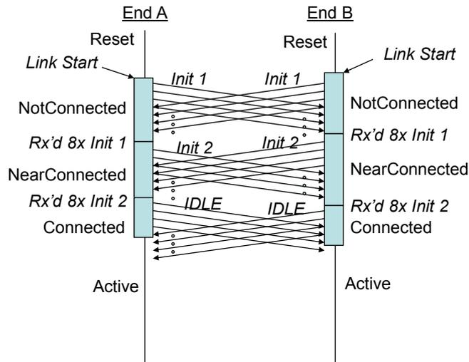
**Figure 3-16: Initialisation when both ends Link Start**
